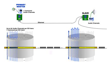
When used within a bi-directional loop, a setting defines whether the audio data is to be read from the down-stream or the upstream.
