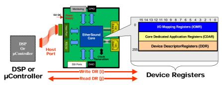
The onboard microcontroller can take care of many non EtherSound tasks such as A/D and D/A management and local HUI.
