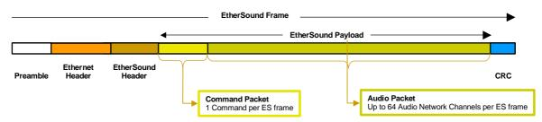
The EtherSound V1 frame has been designed to fully comply with 802.3 in order to allow use of standard Ethernet switches.
