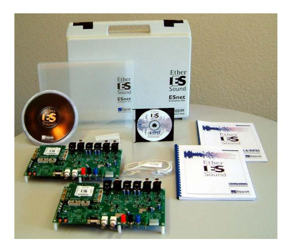
Each Digigram ESnet Evaluation Kit comes complete with two ESnet Evaluation Boards, software and documentation to help you set-up and test a minimum EtherSound environment.
