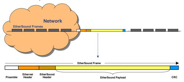
The EtherSound Payload, just like for standard Ethernet frames, is divided in a set of packets. Each packet is made of:
